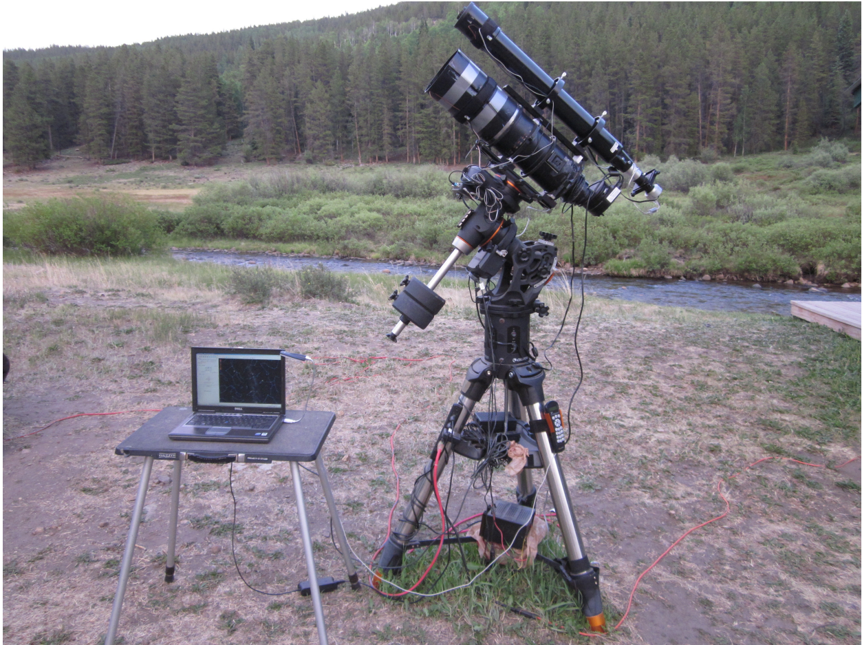
Figure 2.1: Telescope setup showing the guide scope mounted on top of the main scope and controlled by a German equatorial mount. The laptop (left) was used to retrieve and store the images from the main telescope.
