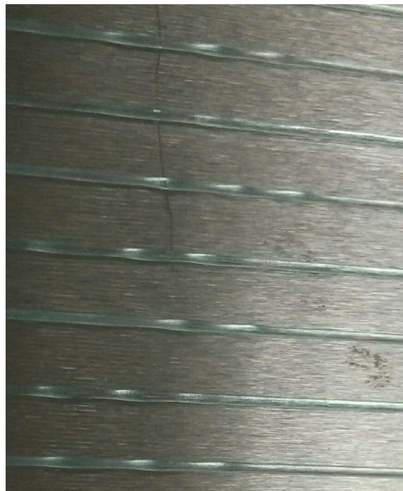
Figure 18: Non-uniform strand width on a brushed aluminum surface
