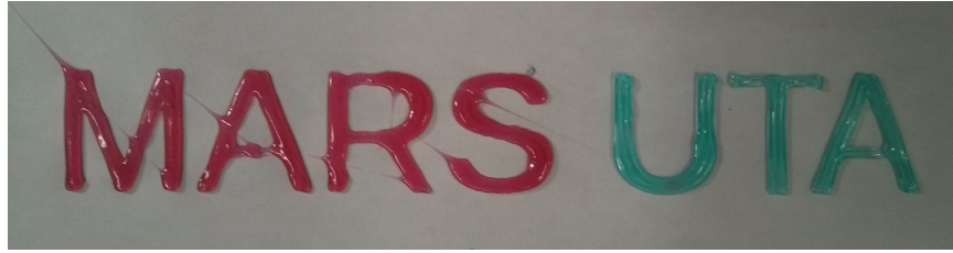
Figure 20: Demonstration of multiple extruders (approximate letter height: 3 cm)
